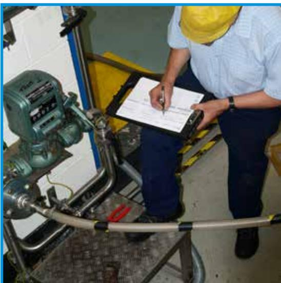
Stream's test rigs are compact and portable and are fully traceable to the highest standards, depending upon the equipment used and the fluids being monitored. The service covers any operationally safe application liquid including food products, solvents, fuel oil and LPG.
